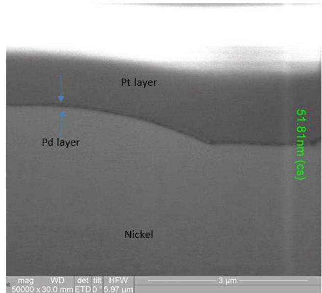
Figure 8: FIB Image of the 6 microinch Electroless Nickel/Electroless Palladium Deposit (50000X Magnification)
