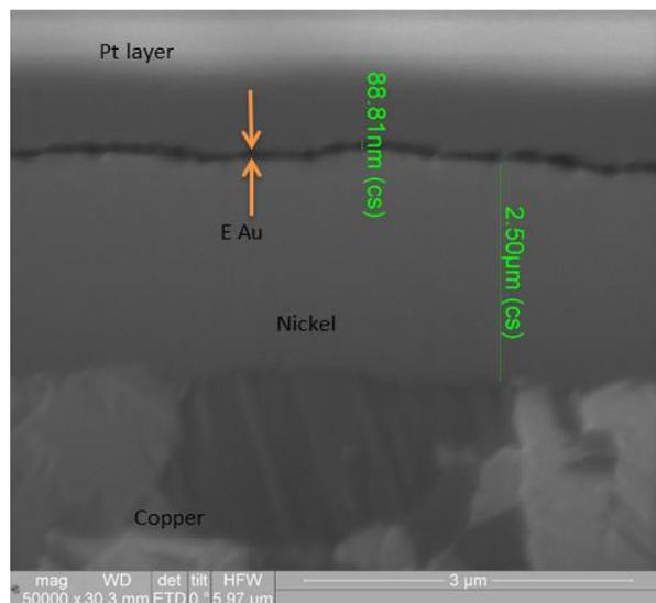
Figure 9: FIB Image of the Electroless Nickel/Electrolytic Gold Deposit (50000X Magnification)
