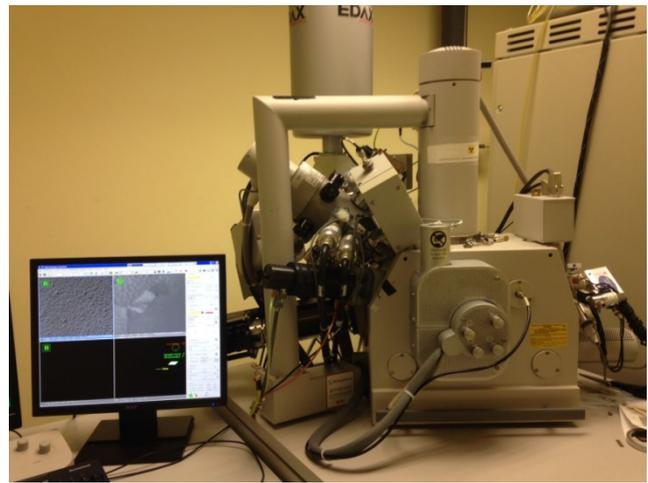
Figure 1: FEI Quanta 200-3A Dual Beam FIB System
