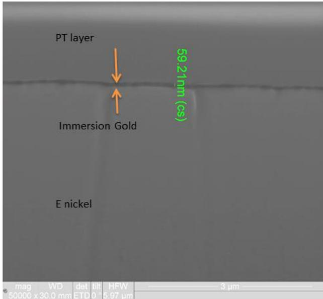
Figure 6: FIB Image of the ENIG Deposit (50000X Magnification)
