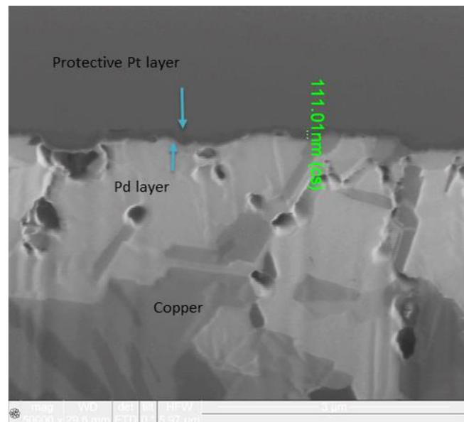
Figure 5: FIB Image of the Nominal 6 Microinch Electroless Palladium Deposit (50000X Magnification)
