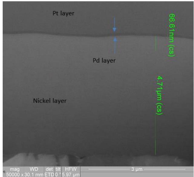
Figure 7: FIB Image of the 3 microinch Electroless Nickel/Electroless Palladium Deposit (50000X Magnification)
