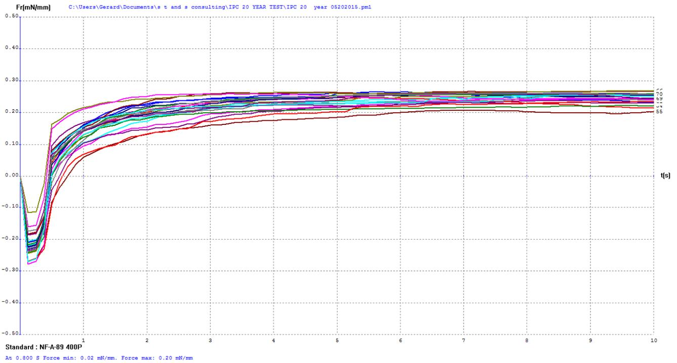
**Figure 15: ENEPIG Test Coupon Wetting Balance Results (3-24 microinch coupons)**
