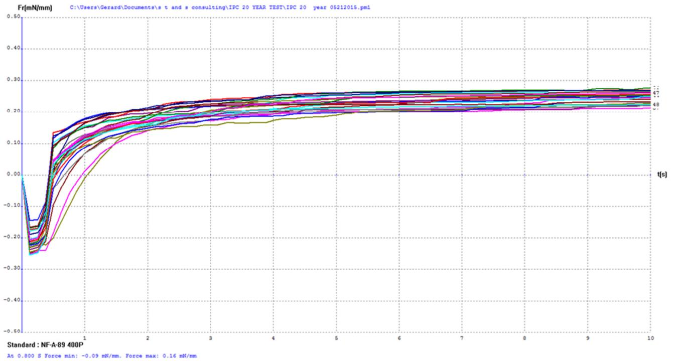
**Figure 16:** Electroless Nickel/Electrolytic Gold Test Coupon Wetting Balance Results
