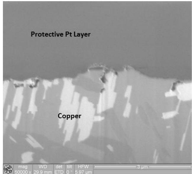
Figure 4: FIB Image of the Nominal 3 Microinch Electroless Palladium Deposit (50000X Magnification)
