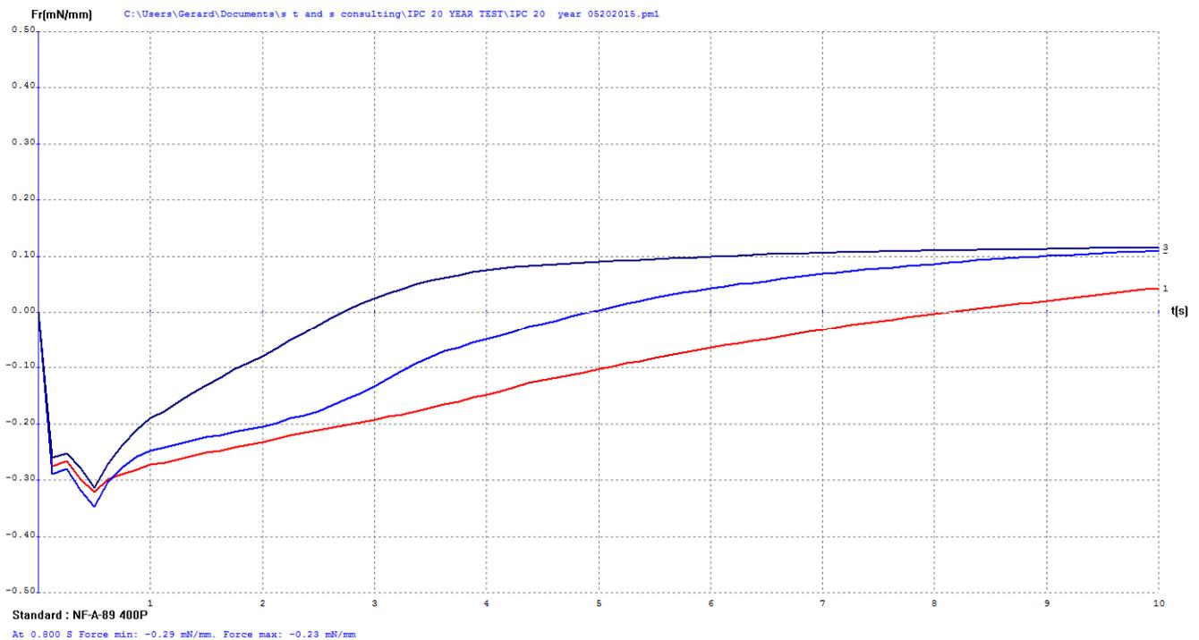
Figure 11: Immersion Silver Test Coupon Wetting Balance Results (3 Individual Test Coupons)
