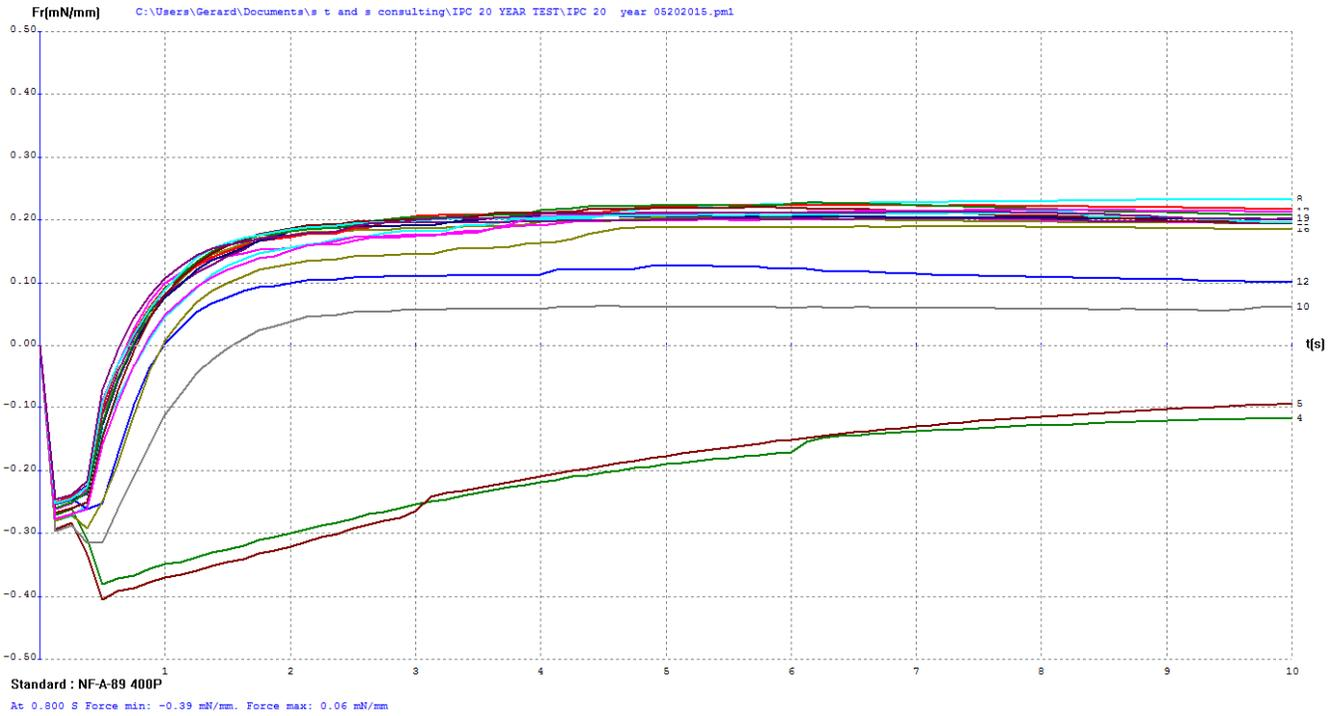
**Figure 12: Electroless Palladium Test Coupon Wetting Balance Results (Test Coupons Covering 3-21 microinch range)**
