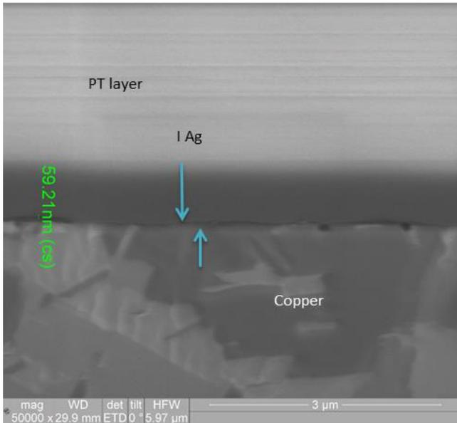
Figure 3: FIB Image of the Immersion Silver Deposit (50000X Magnification)
