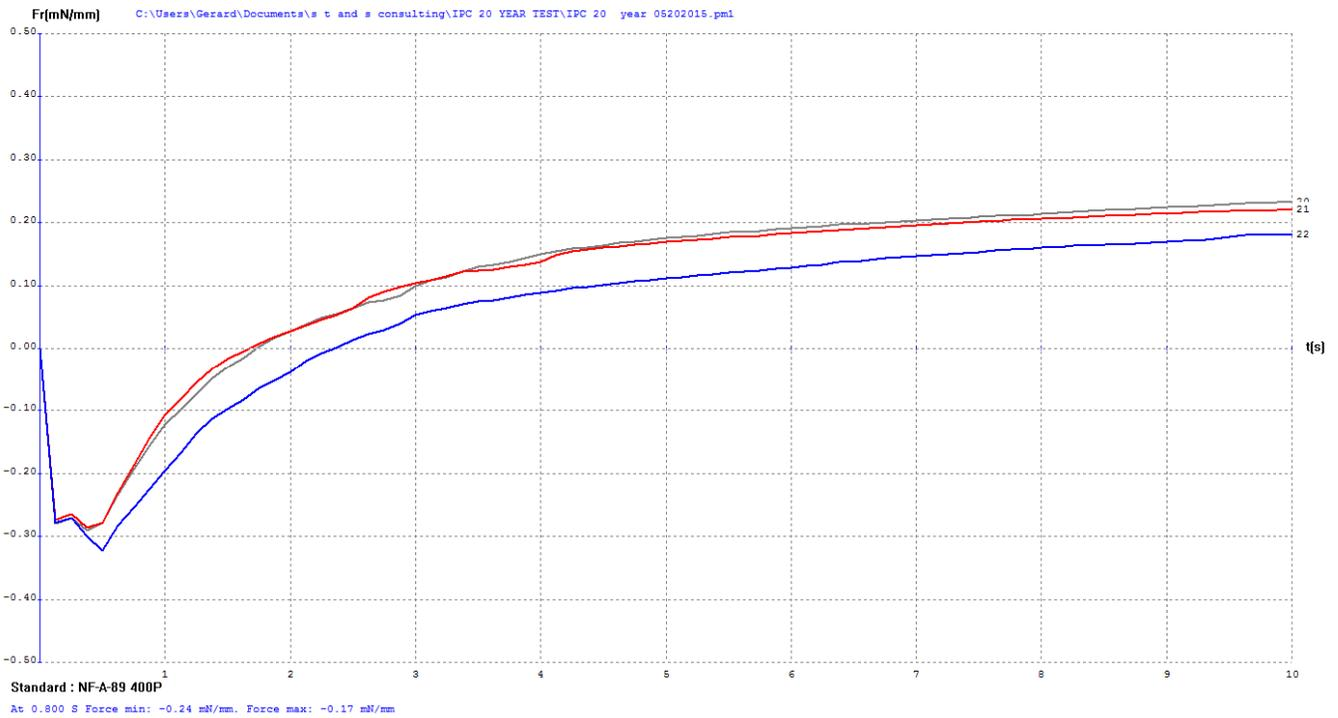
**Figure 13: ENIG Test Coupon Wetting Balance Results (3 Individual Test Coupons)**
