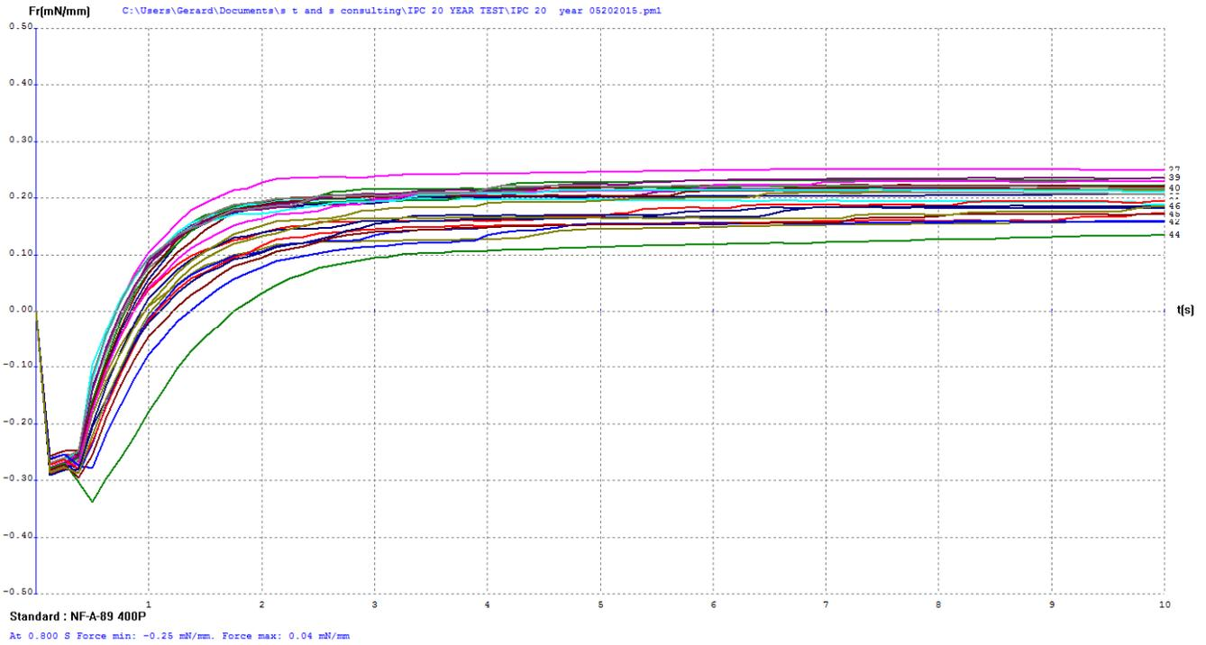
**Figure 14: Electroless Nickel/Electroless Palladium Test Coupon Wetting Balance Results**
