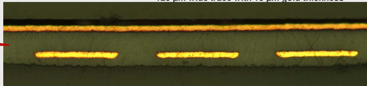
120  $\mu\text{m}$  wide traces with 60  $\mu\text{m}$  spacing in 75  $\mu\text{m}$  thick LCP structure with electrode on top
