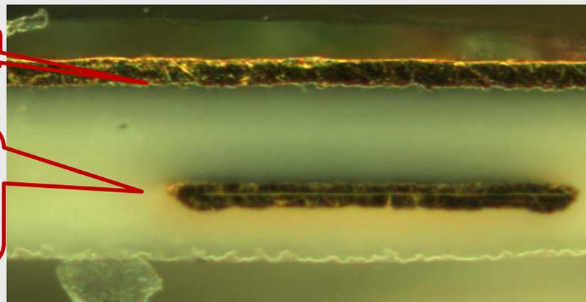
120  $\mu\text{m}$  wide trace with 15  $\mu\text{m}$  gold thickness
