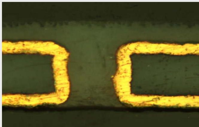
75  $\mu\text{m}$  diameter via with 15  $\mu\text{m}$  gold thickness
