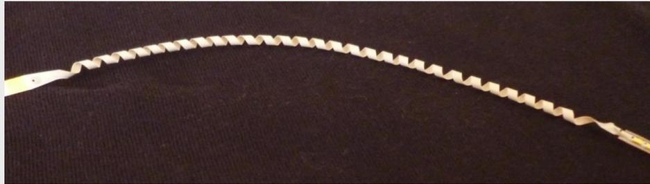
LCP lead structure with electrodes on the surface and embedded metal traces from pure gold
