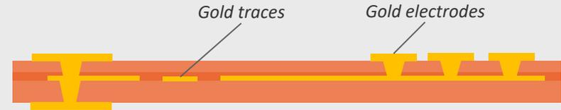
Completely Biocompatible Structure
