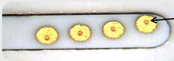
Embedded traces on backside with trace width of 30  $\mu\text{m}$
